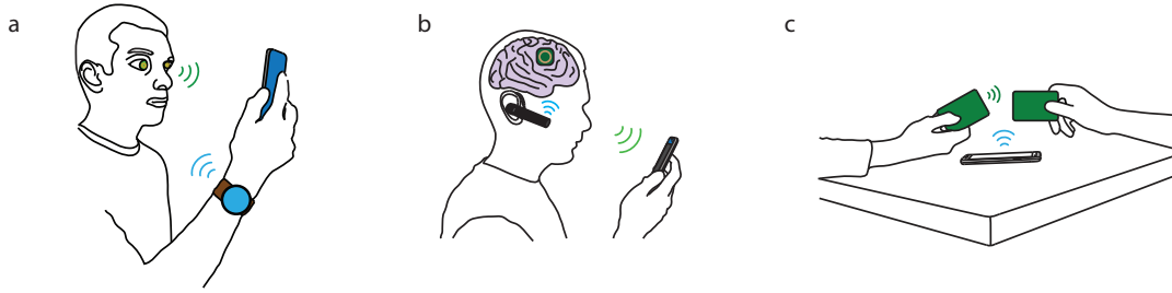
Figure 2—Potential applications of Interscatter communication. (a) Active contact lens systems can backscatter Bluetooth transmissions from a watch to generate Wi-Fi signals to a phone, (b) implantable brain interfaces can communicate by using Bluetooth headsets and smartphones, and (c) credit cards can communicate with each other by backscattering Bluetooth transmissions from a smartphone.
