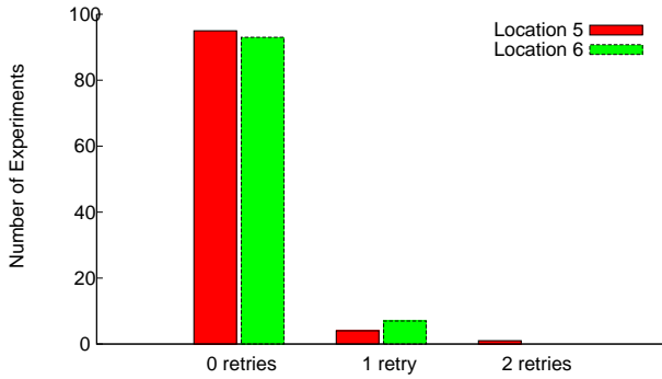
Figure 12—Smart Card Application: The number of retries necessary to successfully communicate between two battery-free smart cards. 94% of tests were successful without any retries.
